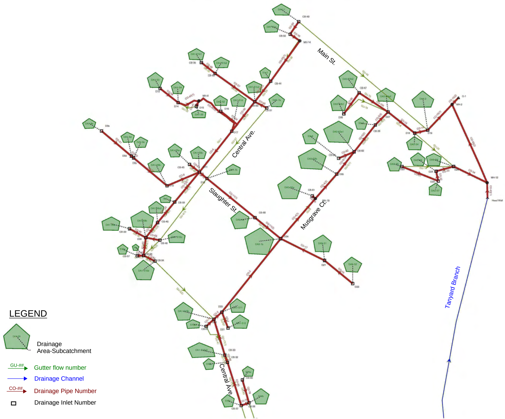
Schematic Diagram - Enlarged Upper Section of Proposed Drainage Network
