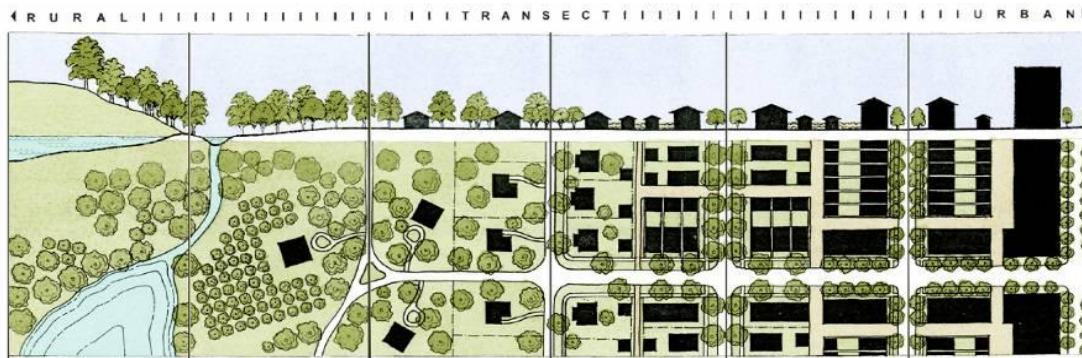
This diagram illustrates how the transect classifies elements of the human environment from rural to urban, in a left-to-right sequence. (Source: Duany, Plater-Zyberk, 2007)
